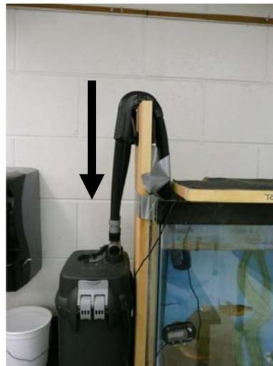
**If you are using the Fluval filter, practice removing the Stop valve and filter top a few times before you install the filter. Remember, the way to open the Fluval filter is to unclip the side clips then using the clip handles, PUSH DOWN on the clip handles. The filter top will pop off.**
